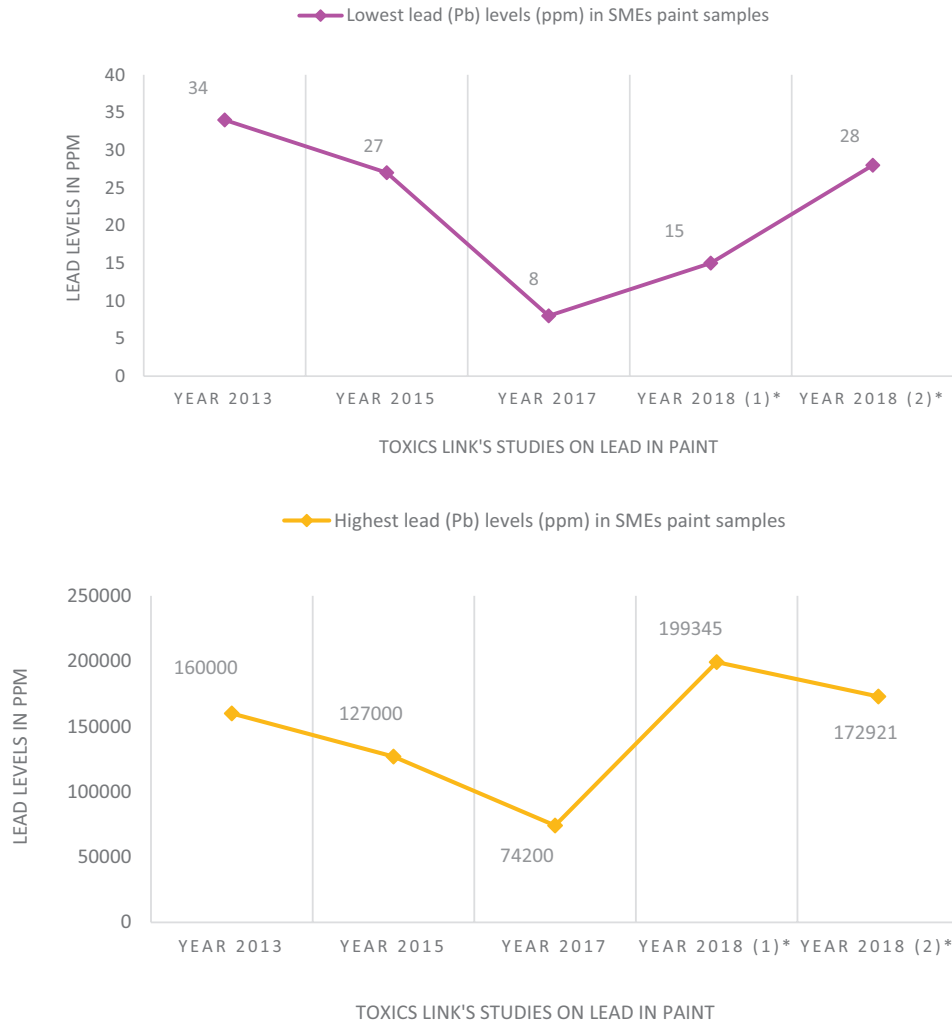
FIGURE 3 TREND OF LEAD CONCENTRATION (IN SMES PAINT) BETWEEN 2013 AND 2018 YEAR 2018 (1) REFERS TO THE SAMPLES ANALYZED IN 2018 STUDY AND MANUFACTURED BEFORE THE REGULATION; YEAR 2018 (2) REFERS TO THE SAMPLES ANALYZED IN 2018 STUDY MANUFACTURED AFTER THE REGULATION
