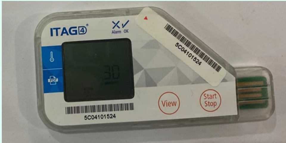
Photo 5: Data loggers are placed in reefers and provide real-time information including temperature
