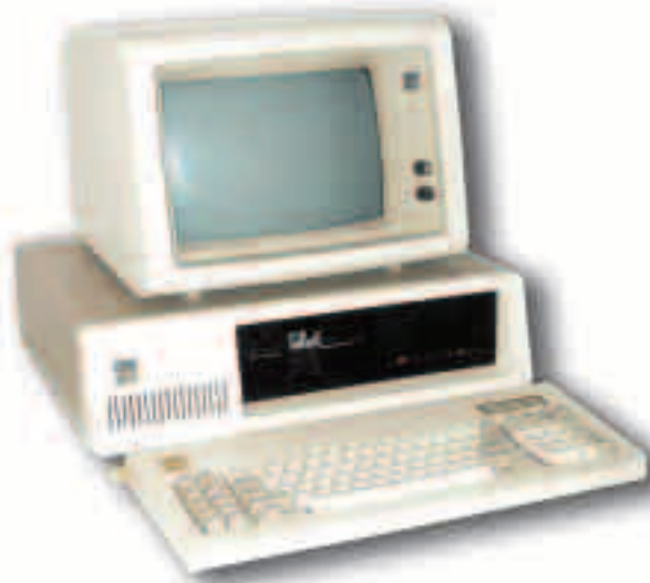
IBM PC XT (1983) - 8086 CPU, 1 MB RAM, 10 MB HD, 4.77 MHz, 16-bit bus, 10 MHz, MS-DOS 1.0
