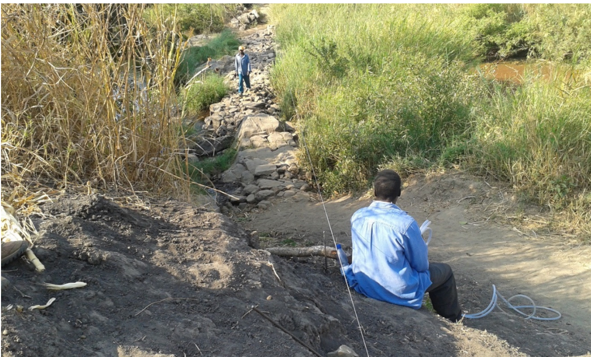
Figure 4: Existing crossing showing line of level survey over raised footpath
