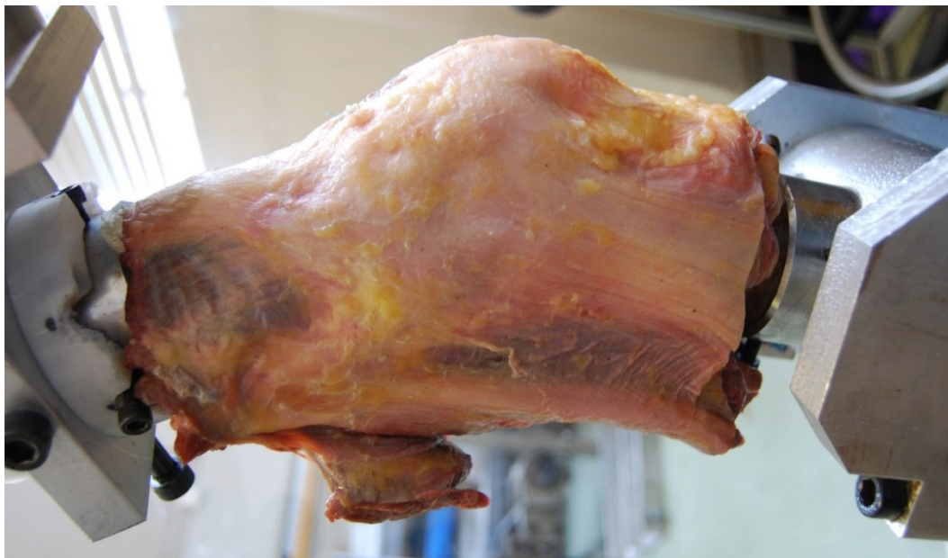
Figure 4.2 Intact-state of the knee mounted into the robot. The femur was attached to the base (right), whereas the tibia was attached to the moving arm of the robot (left)
