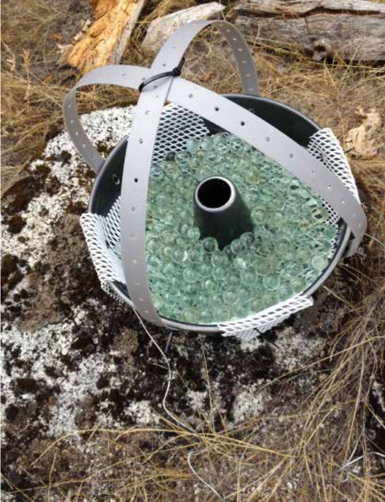
AIR QUALITY monitoring equipment: dust that sticks to marbles can be analyzed later in the lab. Emma Aronson
