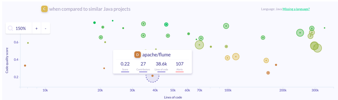
Figure 4: A code quality comparison chart from lgtm.com . The x-axis is LOC and the y-axis is quality. Each bubble is an open-source Java project. The highlighted project, apache/flume , has 107 alerts, a quality score of 0.22 and final grade D.
