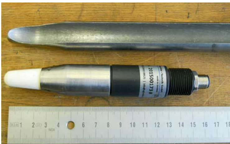
Figure 2: Suction probe and special drill bit.
