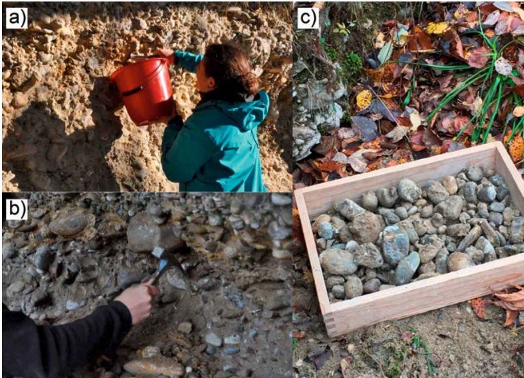
Figure 3: Pictures from the site Irchel a) Clast collection for the petrography at Scharfenflue. b) collecting vein-quartz-clasts for the clast morphometry at Hasli. c) collected clasts in the sieve for the clast petrography at Hochwacht.
