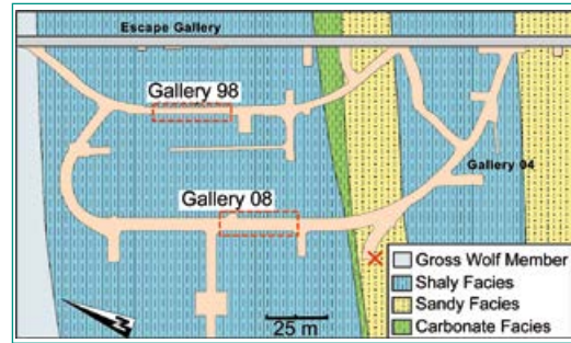
Figure 1: Location of the SE-P project experiment sites, gallery 08 and gallery 98. The two galleries are aligned normal to bedding strike, but have different sizes and ages (about 10 vs. 20 years). The Mont Terri URL layout figure was modified after Kaufhold et al. (2016).
