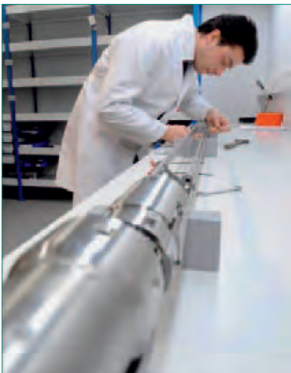
Fig. 2: Test rig fabrication in the Halden instrument workshop.
