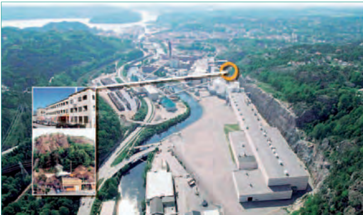
Fig.1: The Halden Boiling Heavy Water Reactor is located in a rock cavern in the city of Halden, South-East Norway. The reactor also provides steam to the paper factory next-door.
