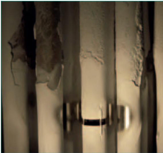
Figure 1: Aerosol deposit layer on the surface of the bundle tubes close to the tube break after Test B12.
