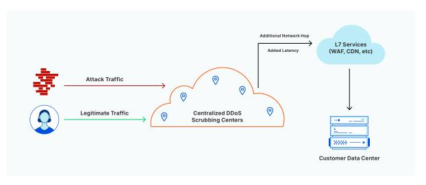
'Scrubbing centers' are distant and few and dedicated to DDoS mitigation. This requires network traffic to travel to an alternate data center for any additional L4-7 processing incurring additional delay.
