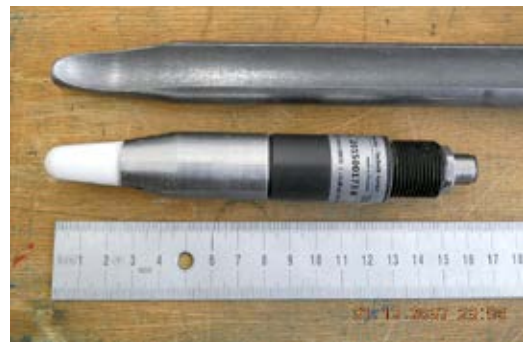
Figure 2: Suction probe and special drill bit.
