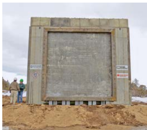
Figure 4: Test Slab, Reinforced Concrete Supporting Structure, Steel Frame Set-up No. 1 (Tests 1&2)
