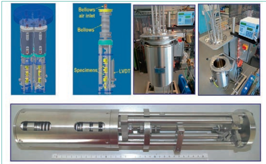
Figure 3: Servo-pneumatic bellows-loading system and autoclave for SCC initiation tests.
