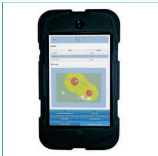
Figure 4: Work Plan and 2D Dose Map from the Halden Planner shown on a robust Handheld Device.
