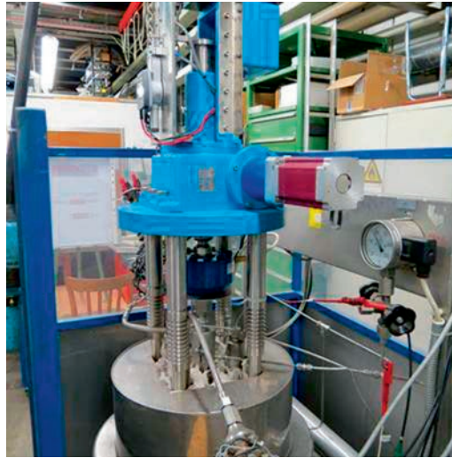
Figure 1: New electro-mechanical loading system for EPFM tests in high-temperature water.
