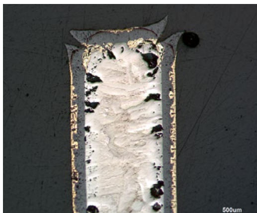
Figure 4: Vertical cut of cladding sample with 10 minutes pre-oxidation and 30 minutes nitriding at 1100 °C
