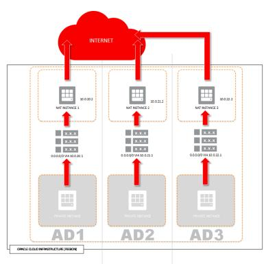
In the case of a NAT gateway failure, traffic should fail over to the NAT gateway in the other Availability Domain as shown in the following diagram:
