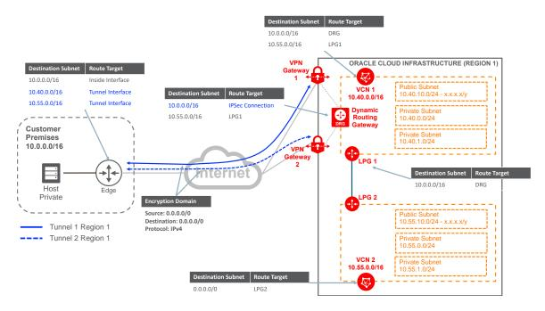
Figure 10. Routing for VPN Connect for the Same Region with Multiple VCNs with a Single Customer Edge Device
