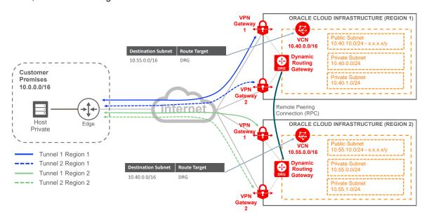
Figure 12. VPN Connect for Dual Regions with a Single Customer Edge Device Routing
