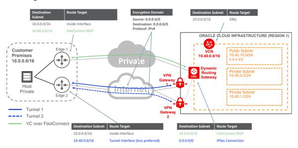
Figure 7. Routing for FastConnect Plus a Single Region and a Single Customer Edge Device VPN
