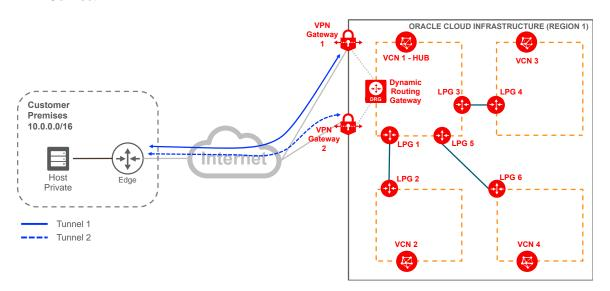
Figure 8. VPN Connect for the Same Region with Multiple VCNs—High-Level Design
