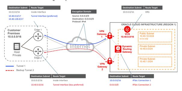
Figure 5. Routing and Encryption Domain for VPN Connect for a Single Region with Redundant Customer Edge Devices
