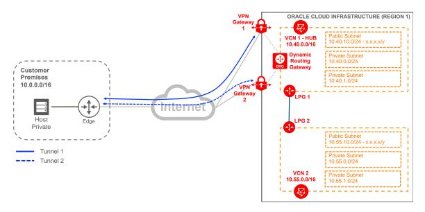
Figure 9. VPN Connect for the Same Region with Multiple VCNs with a Single Customer Edge Device
