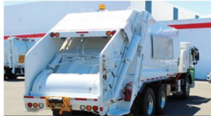
REAR LOADER 295 kWh battery capacity 65 MILES per charge Used for the residential Clean Up Day program
