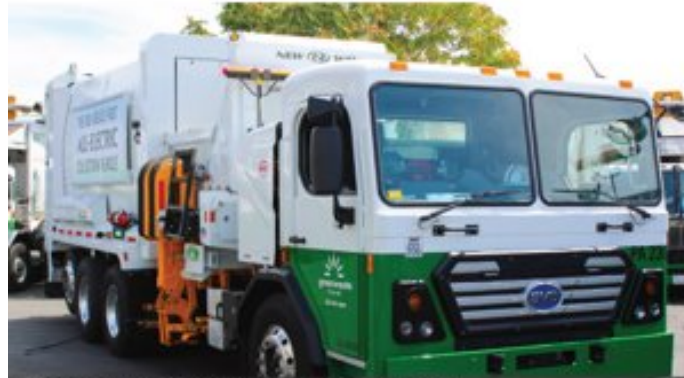
FULLY AUTOMATED SIDE LOADER 295 kWh battery capacity 50 MILES per charge Used for residential garbage collection
