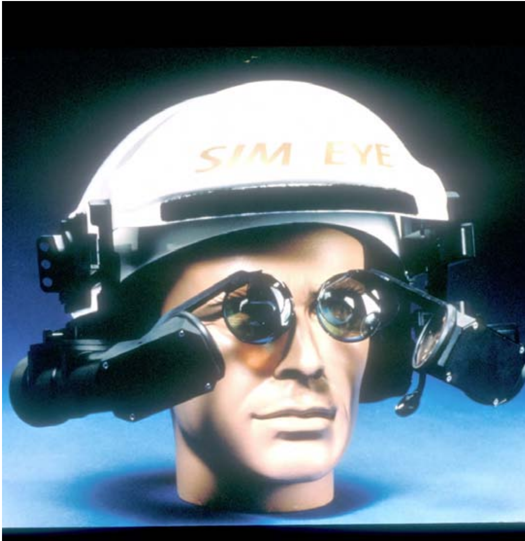
A SimEye helmet-mounted virtual display (Ben Delaney)
