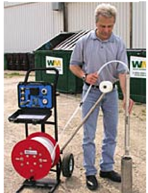
Low Flow Double Valve Pump Setup in Field
