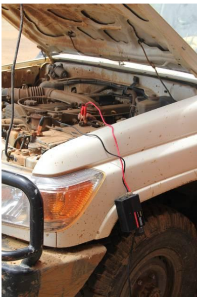
The use of power inverters instead of a generator to operate the microscopes (far cheaper and less maintenance)
