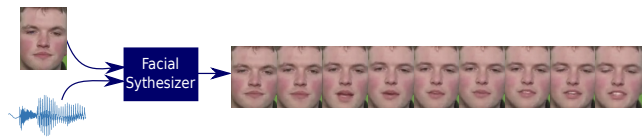
Figure 1: The proposed end-to-end face synthesis model, capable of producing realistic sequences of faces using one still image and an audio track containing speech. The generated sequences exhibit smoothness and natural expressions such as blinks and frowns.
