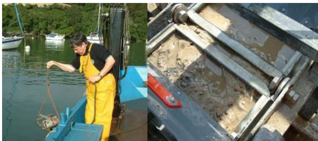
Figure 4.2A: Mini van Veen sampler being deployed; 4.2B: Close up of a sample collected from Mylor Harbour.
