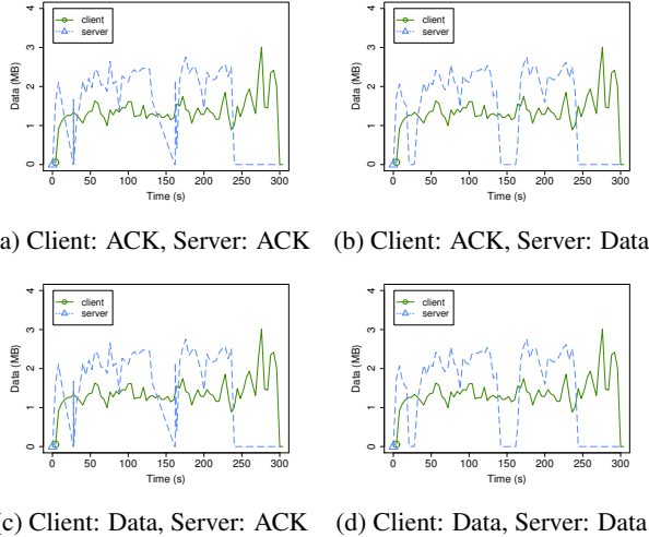
Figure 5: Asymmetric traffic analysis shows low correlation between an unmatched client/server pair
