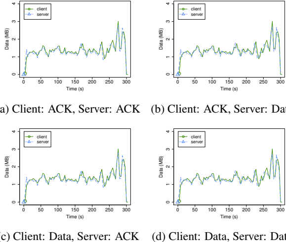
Figure 4: Asymmetric traffic analysis shows high correlation between a matched client/server pair
