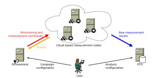
Figure 1: Schematic representation of the complete measurement architecture.
