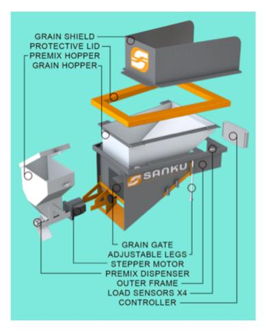
With its "universal mill" design, installation is quick and seamless with no need to modify the existing mills technology. Furthermore, minimal training is required due to the dosifier being fully automated, causing little or no disruptions to the established daily routine of the miller.
