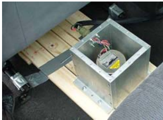
Fig.5 - LN-200 IMU mounted on to the IMU-Bench prototype.
