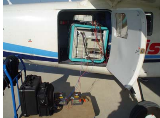
Image 7: The TAG inside the airplane with batteries supply for the static data acquisition phase.
