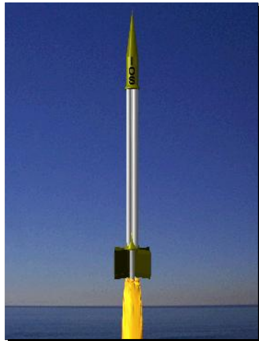
Figure 9.1: The Interorbital Systems RSX-2 rocket. The RSX-2 is capable of lifting a 5 pound payload into the upper atmosphere using four liquid-fueled thrusters. It is the only liquid-fueled sounding rocket in production. Such rockets are desirable because of their low acceleration rates and non-corrosive exhaust products.
