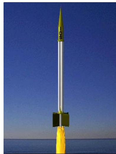
Figure 1.1: The RSX-2 Rocket of Interorbital Systems, Inc. Without fins the RSX-2 would be unstable. Developing an active guidance system for a finless version of the RSX-2 is a challenging problem, and the subject of chapter 9.
