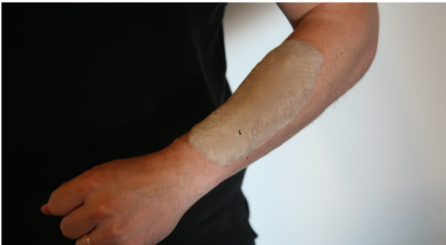
Figure 16. Artificial skin, created from silicon, covered the 3in3out device to simulate implantation and allow for testing.
