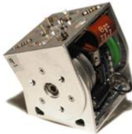
Figure 4. Mark Yim's third generation Polybot module
