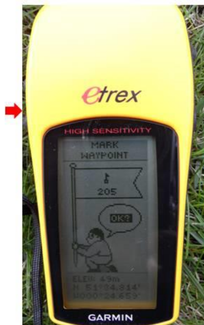
Step 7. Press again ENTER key to save in memory the new waypoint
