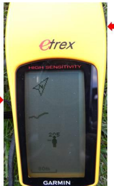
Step 8. Press PAGE key to view the new location in the Map screen
