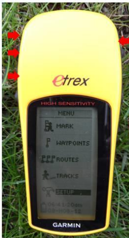
Step 1. Press PAGE key to select Menu page and use UP/DOWN keys to highlight Setup menu.
