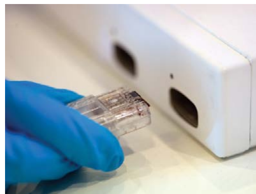
The semi-conductor microchip being inserted into the DNA analyser.
