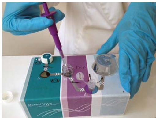
A prototype DNA test kit, incorporating a semi-conductor minilab, that allows 'live' DNA testing.
