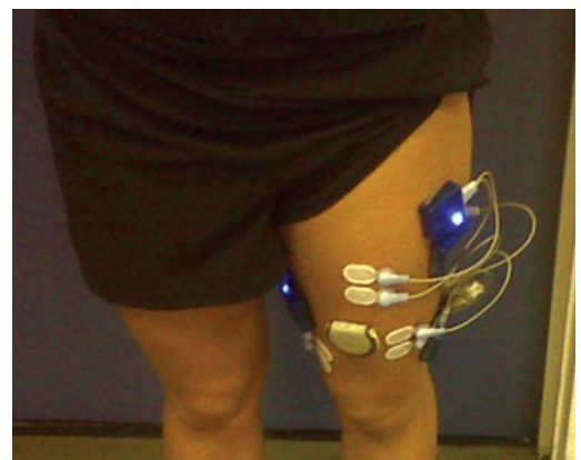
Figure 2. Wireless EMG sensors. Electrodes attached to leg muscles VL and VM.
