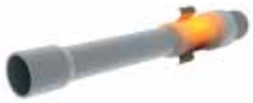
12. Heating and heat treatment of weld area
