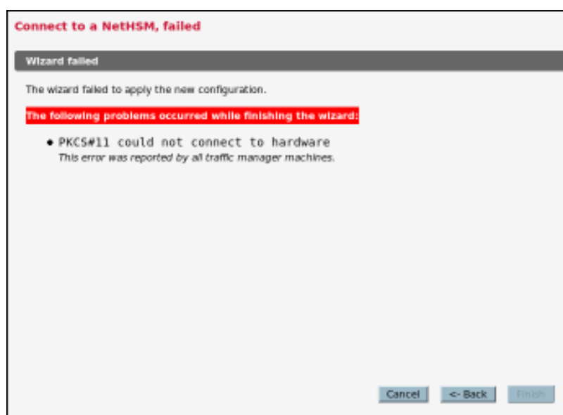
Fig 50. Reporting of connection failures
