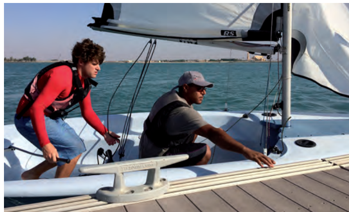
With the wind blowing away from the pontoon at 45° - a ¾ tack positions the boat perfectly alongside with sails de-powered
