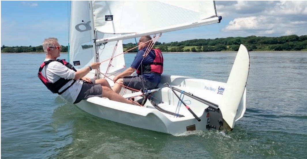
Make sure the blade is clear of the water and lift the centreboard a little
