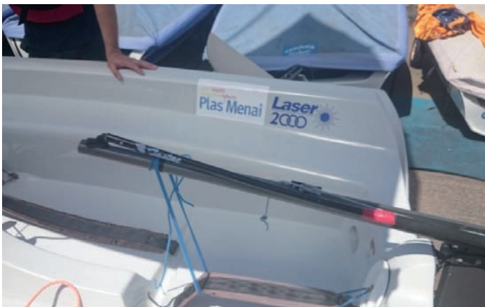
If the boat is hard to turn move the bungee backwards or ease the tension
