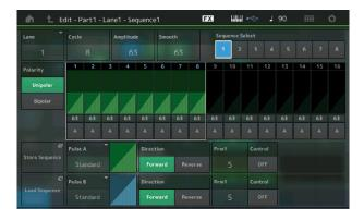
The number of Steps can be set with the parameter "Cycle". The default setting "Cycle = 8" offers eight Steps.
