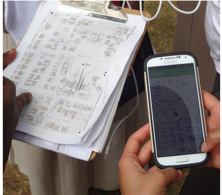
Dzivarasekwa, Zimbabwe - Volunteers using the OpenMapKit App and Field Papers to collect data on each house.
