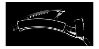
The patented Rolex Glidelock fine adjustment system allows divers to adjust the length of the bracelet for a secure and comfortable fit over a diving suit, without using any tools. A robust toothed panel under the clasp cover provides an extension of up to 20 mm in 2 mm increments.
