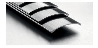
Rolex uses 904L stainless steel for its steel watch cases. 904L is mainly used in the high technology, aerospace and chemical industries, where maximum resistance to corrosion is essential. A superalloy, 904L is extremely resistant and highly polishable. It maintains its beauty even in the harshest environments. 904L steel also provides a perfect complement to the precious metals used by Rolex.
