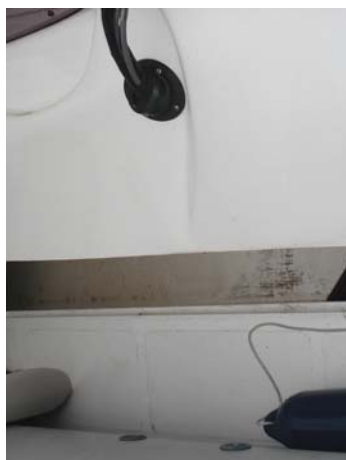
Console only secured by four self tapping screws along small 'ledge'
