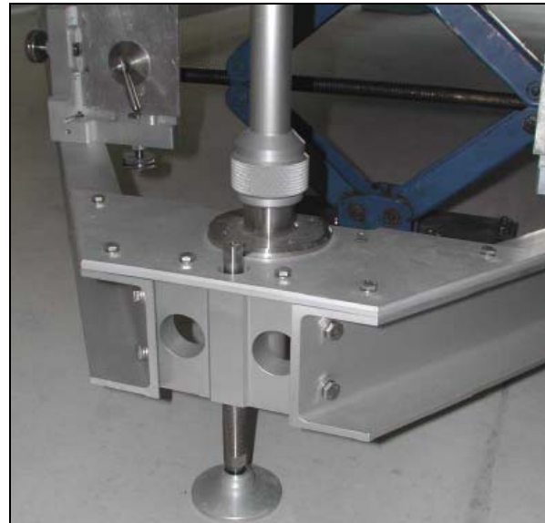
The template clamp, fine adjustment system, precision alignment line and levelling feet used to precisely position the templates so that they are vertical and in the section planes.
