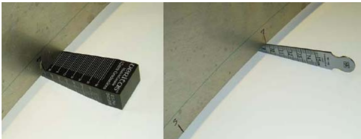
Figure 9.3.8 Wedge gap measurement
