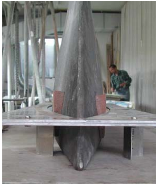
Demonstration of keel template measurements. The templates are pinned together and supported by three pillars at a precise height above the base plane. They can then be easily aligned and wedged in place for gap measurement. The actual measurements are made on the finished keel, not the casting as shown here.
