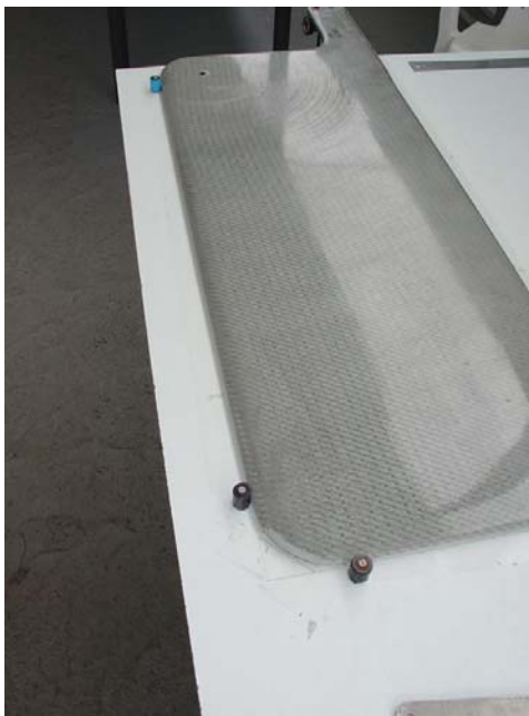
Left, 420 Centreboard template prepared for event inspection on melamine coated surface, and right, detail from a 470 rudder template. Both classes are using a similar system to define their measurement axes, with the origin point at the intersection of the leading and bottom edges.
