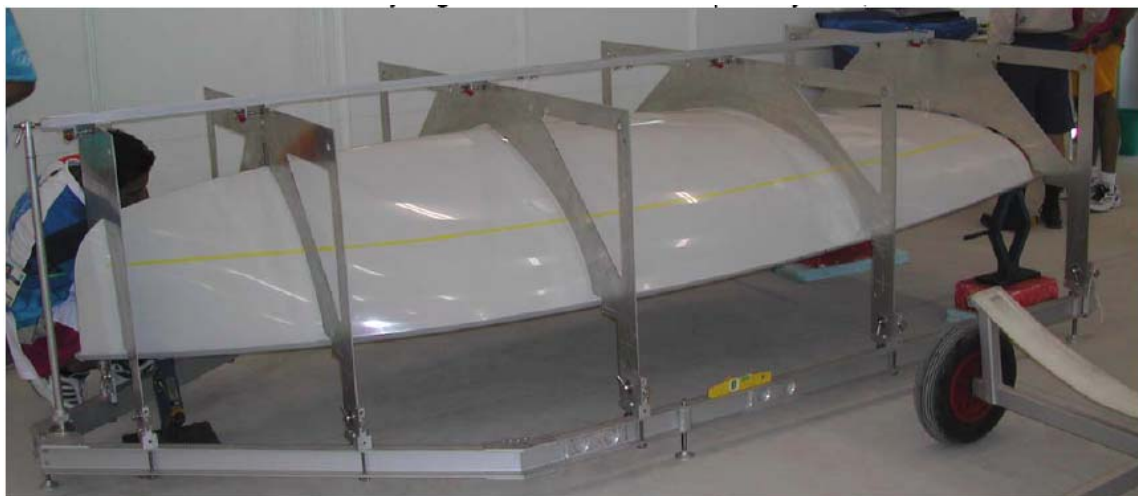
The Europe hull inside the jig, levelled and aligned using car jacks
