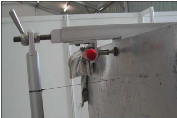
The template clamp, fine adjustment system, precision alignment line and levelling feet used to precisely position the templates so that they are vertical and in the section planes.
