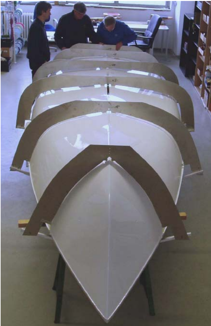
Left, a Flying Dutchman hull with the templates positioned relative to the hull.
