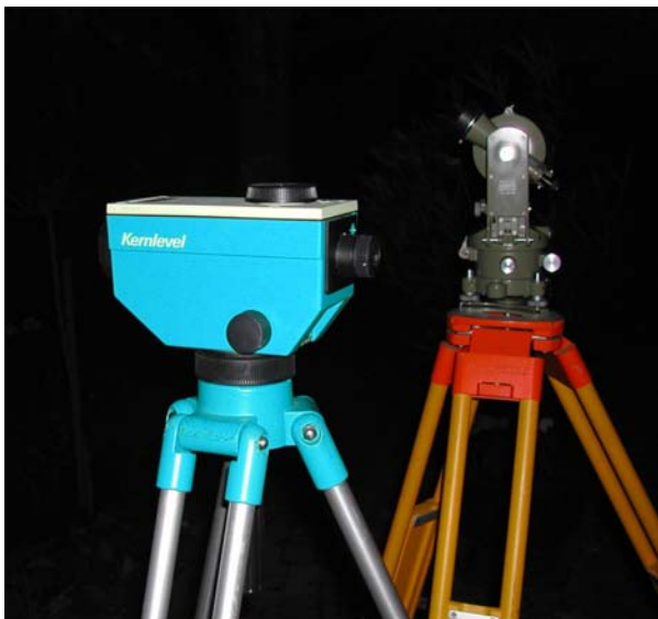
Figure 8.3.8 a - Surveyor's level and theodolite
