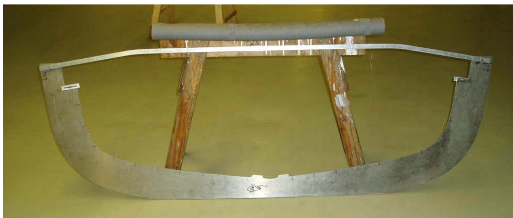
Figure 9.3.3 A full section FD template made of Dural with a pinned rigid crossbar and adjustable lugs at the sheer, for alignment. However, again there is no reference line at 10 mm from the template edge. The signature shows that this template has been checked against the Mylar plan.
