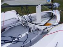
Remove the dagger board and ensure it fits in the dagger slot.
