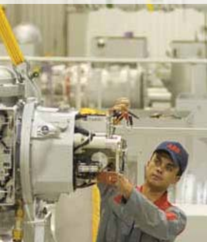
Switchgear is a little like the fuse box in your house only much larger, containing fuses and circuit-breakers.
