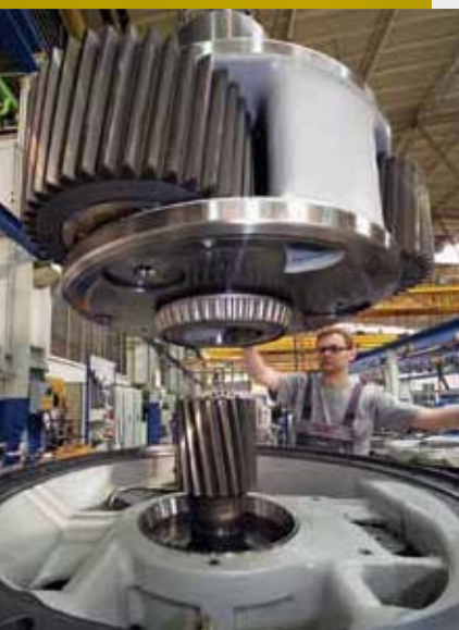
Assembly of a wind turbine gearbox.
