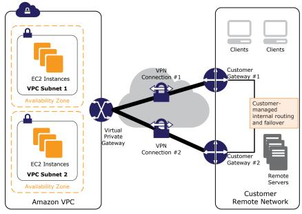
Figure 2 – Redundant Hardware VPN Connections
