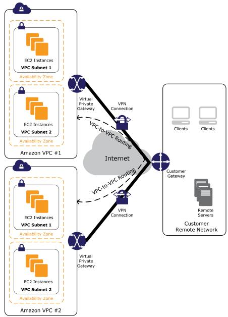
Figure 10 - Routing Traffic Between VPCs
