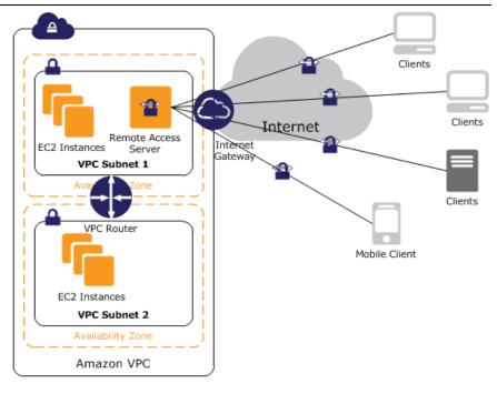
Figure 12 - Remote Access Solution
