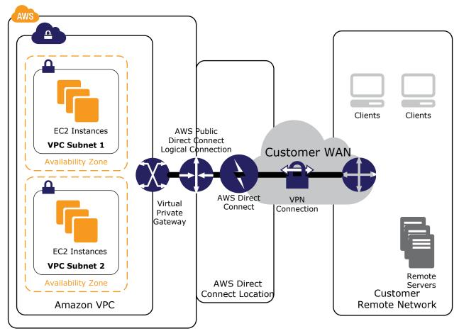
Figure 4 - AWS Direct Connect + VPN
