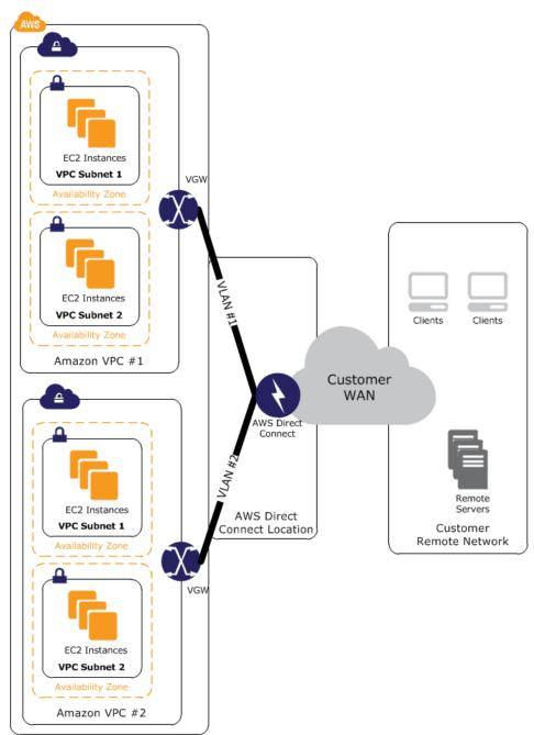
Figure 11 – Intra-Region VPC-to-VPC Routing with AWS Direct Connect
