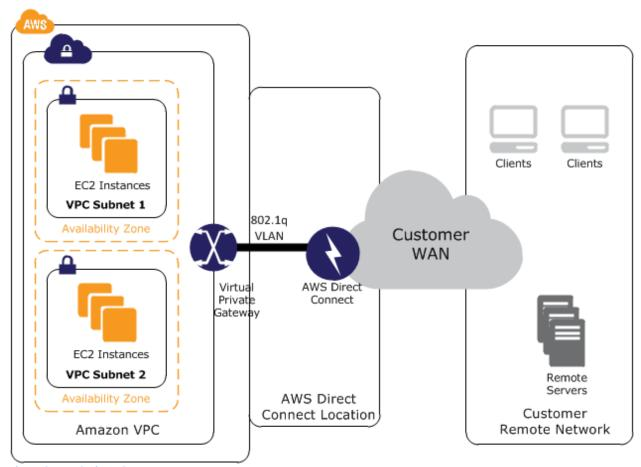
Figure 3 – AWS Direct Connect
