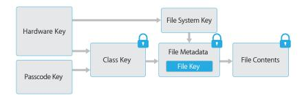
The content of a file is encrypted with a per-file key, which is wrapped with a class key and stored in a file's metadata, which is in turn encrypted with the file system key. The class key is protected with the hardware UID and, for some classes, the user's passcode. This hierarchy provides both flexibility and performance. For example, changing a file's class only requires rewrapping its per-file key, and a change of passcode just rewraps the class key.
