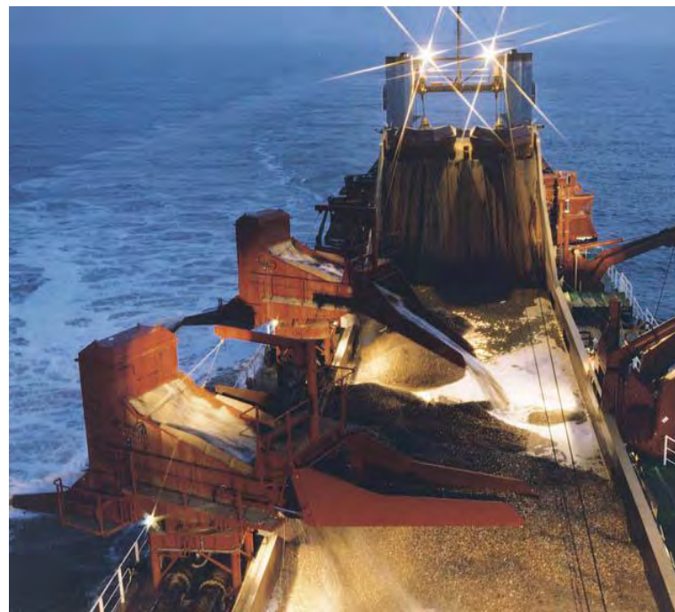
Figure 13.2: Screening of marine aggregates on board a trailer suction hopper dredger (photo courtesy British Marine Aggregate Producers Association).
