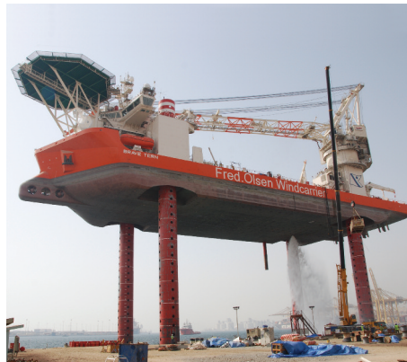
Brave Tern undergoes a jack-up test.
