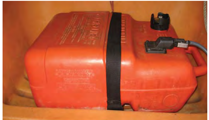
Fuel tanks and batteries should always be strapped down.
