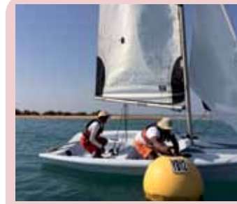
Assuming no tidal flow, aim to pick up the mooring by the windward shroud.
